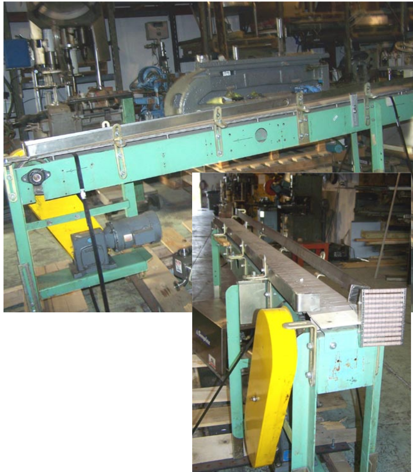
Hytrol Conveyor, 6"W x 96"L, 1/2hp, 3ph, Option: add $250 for variable speed inverter
