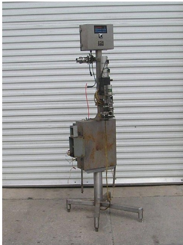
Scholle Autofill 9P, pneumatic & electric cut off fill device (photo prior to reconditioning process)
